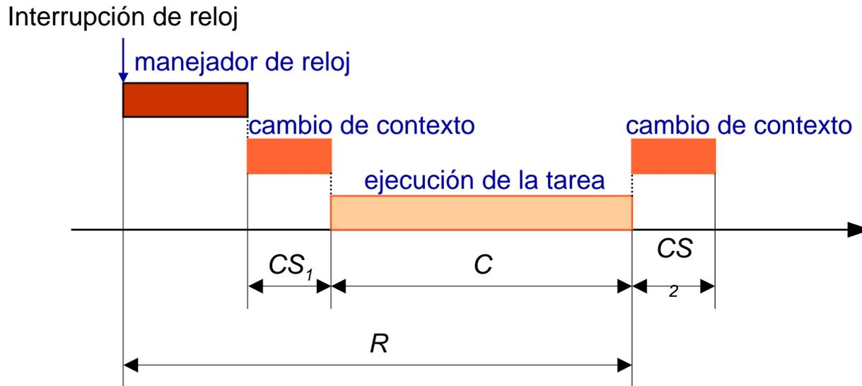
$$R_i = CS_1 + C_i + B_i + \sum_{j \in hp(i)} \left\lceil \frac{R_i}{T_j} \right\rceil \cdot (CS_1 + C_j + CS_2)$$
